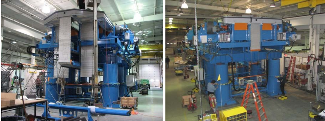
Figure 8.9: Independent 4WD chassis dynamometer undergoing shop tests.
