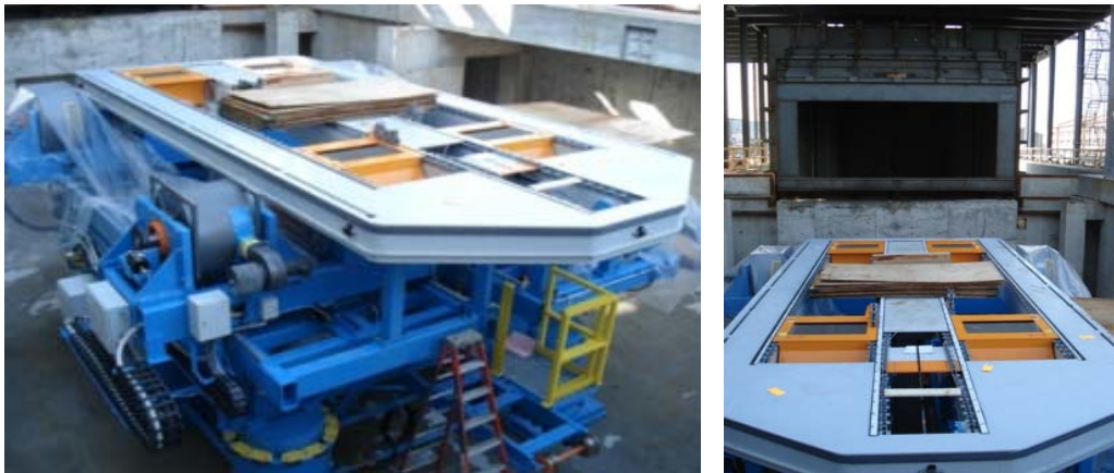
Figure 8.12: Independent 4WD chassis dynamometer with moveable base sitting in basement on site. Test section floor is yet to be installed.
